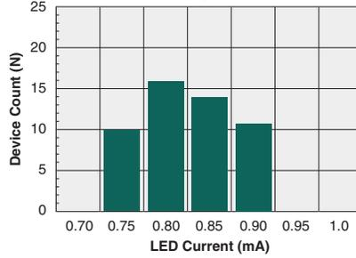
**Typical  $I_F$  for Switch Dropout**
