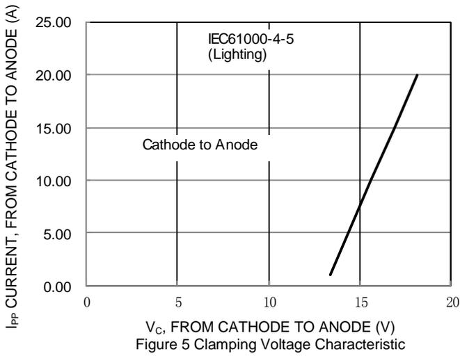
Figure 5 Clamping Voltage Characteristic
