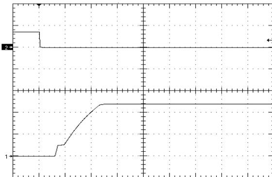
Figure 7. Startup Waveform via Enable Pin, time scale 10mS/div. Vin=Vin\_nom, no load negative enable, Ch1=5V/div, Ch2=5V/div
