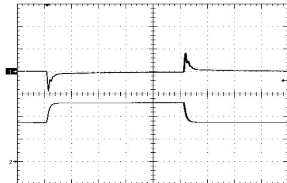
Figure 10. Load Transient Response (100mV/div), di/dt=0.1A/uS, 50% - 75% - 50% of full load, time scale: 200uS/div Ch1=100mV/div, Ch2=2A/div
