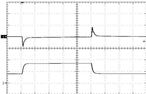
Figure 9. Load Transient Response di/dt=0.1A/uS, 25% - 50% - 25% of full load, time scale: 200uS/div Ch1=100mV/div, Ch2=2A/div
