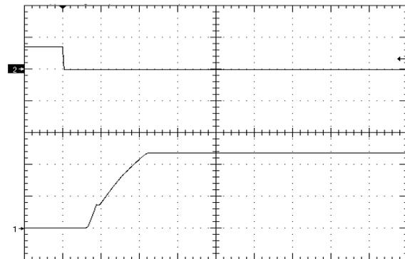
Figure 8. Startup Waveform via Enable Pin, time scale 10mS/div. Vin=Vin\_nom, full resistive load + 3300uF, Ch1=5V/div, Ch2=5V/div
