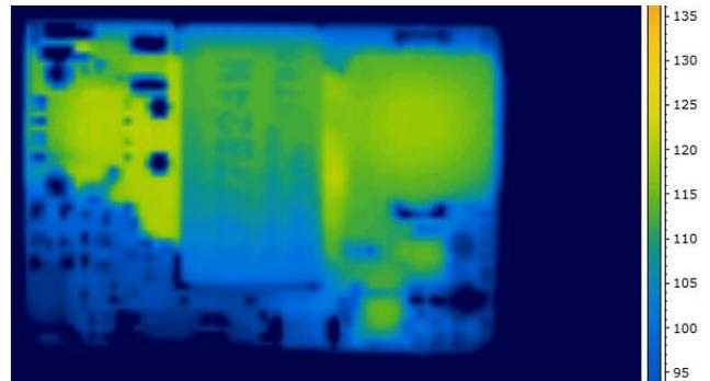
Figure 4. Thermal Image of CPT7B24 7A output, 45C Ambient, 200LFM, Vin = 24V, airflow from pin 3 to pin 1, T<sub>max</sub> = 123°C
