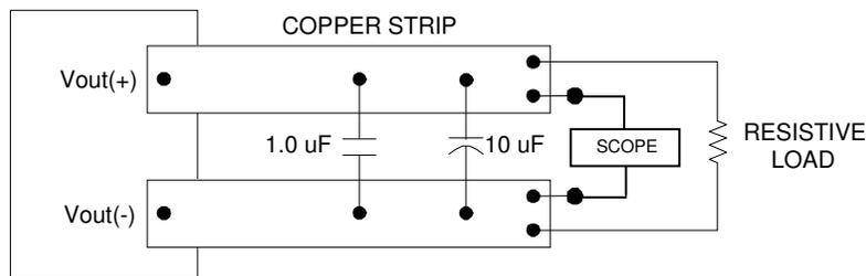
Note: Use a 1.0 $\mu\text{F}$  X7R ceramic capacitor and a 10 $\mu\text{F}$  @ 25V tantalum capacitor. Scope measurement should be made using a BNC socket. Position the load 3 in. [76mm] from module.
