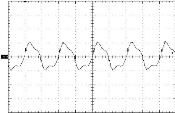
Figure 5. Output Voltage Ripple (20mV/div), time scale - 1uS/div. Vin=Vin\_nom, full resistive Cout=1uF ceramic + 10uF Tantalum (see Fig 12)
