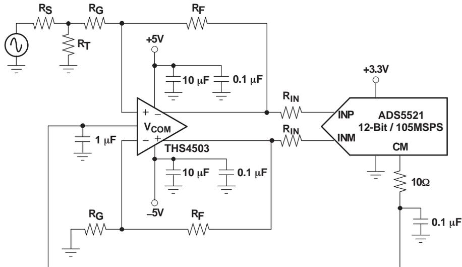
Figure 42. Using the THS4503 with the ADS5521
