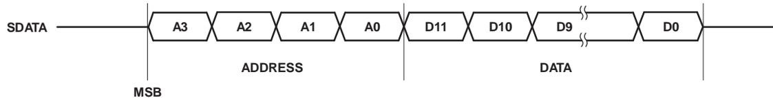
Figure 3. DATA Communication is 2-Byte, MSB First
