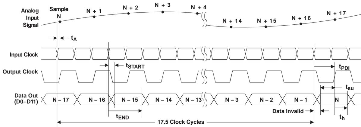
A. It is recommended that the loading at CLKOUT and all data lines are accurately matched to ensure that the above timing matches closely with the specified values.
