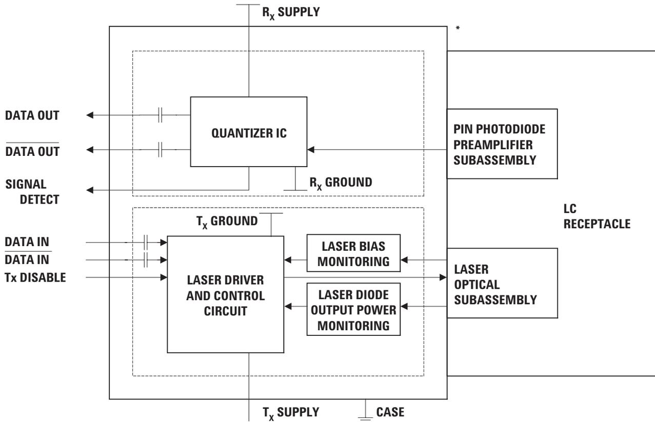
\* NOSE CLIP PROVIDES CONNECTION TO CHASSIS GROUND FOR IMPROVED EMI PERFORMANCE
