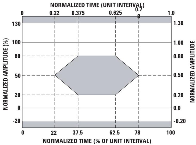
Figure 9. Gigabit Ethernet Transmitter eye mask diagram
