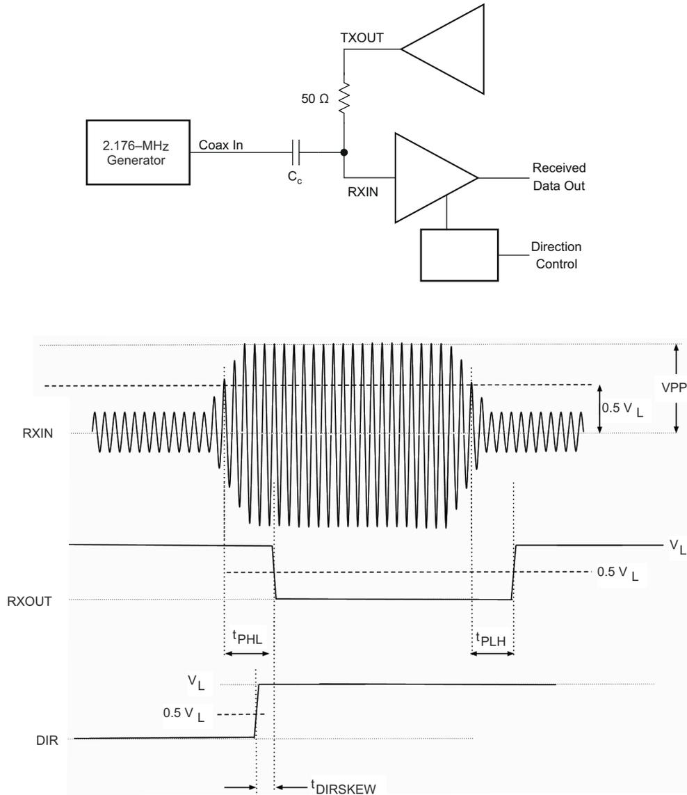
**Figure 7-2. Measurement of Modem Receiver Propagation Delays**
