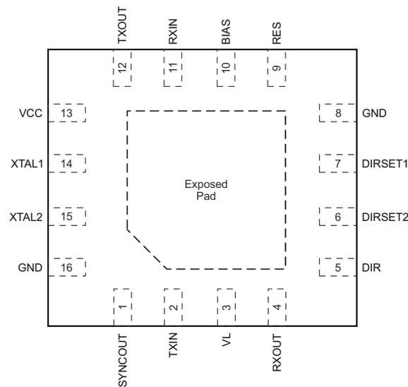
**Figure 5-1. RGT Package, 16-Pin VQFN, Top View**
