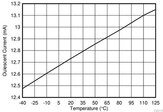
**Figure 6-11. Supply Current vs Temperature in Standby Mode**
