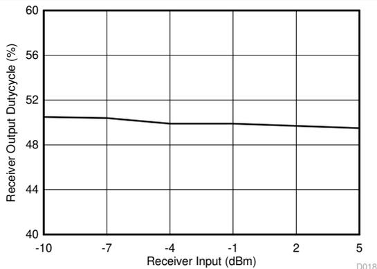
**Figure 6-17. Receiver Duty Cycle With 9.6 kbps Signaling Rate**
