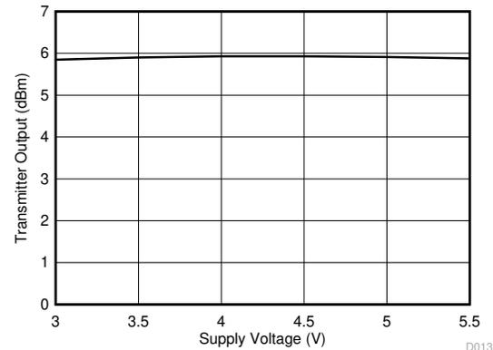
**Figure 6-12. Transmitter Output Power vs Supply Voltage**
