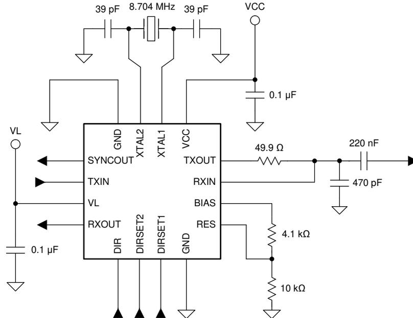
Figure 9-3. SN65HVD64 Schematic
