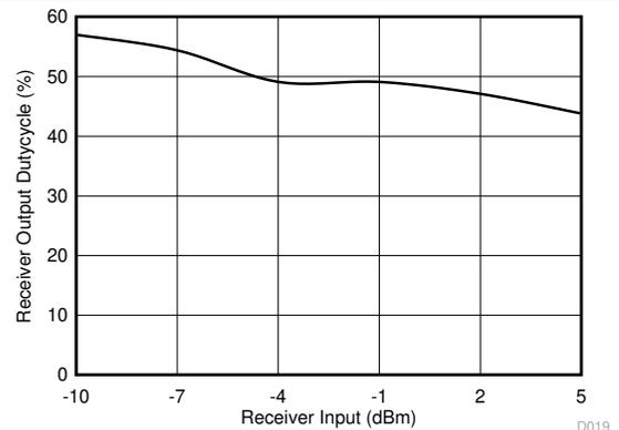
**Figure 6-18. Receiver Duty Cycle With 115.2 kbps Signaling Rate**
