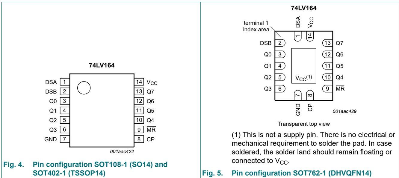
Fig. 4. Pin configuration SOT108-1 (SO14) and SOT402-1 (TSSOP14)
