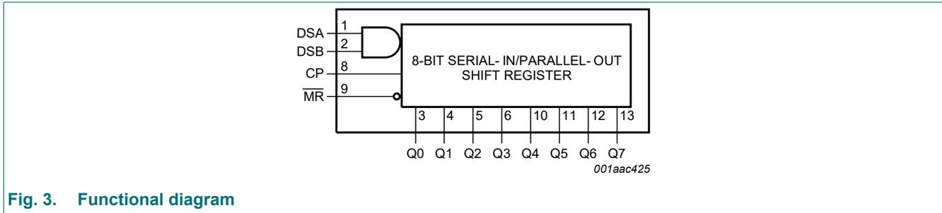
Fig. 3. Functional diagram
