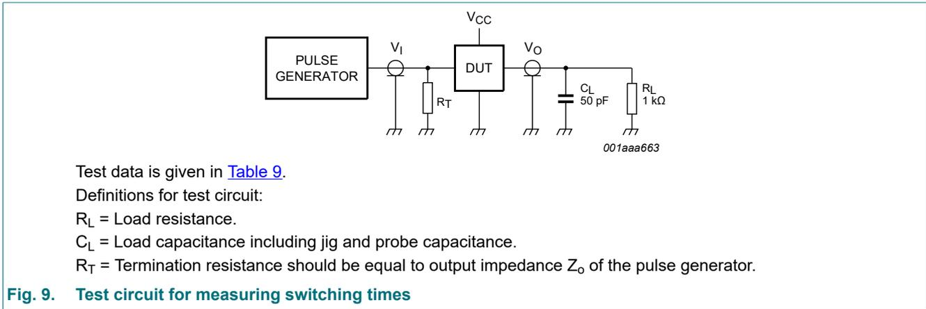
**Fig. 9. Test circuit for measuring switching times**
