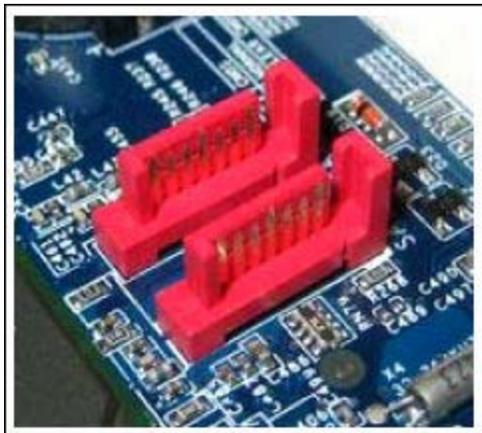
Figure 1. SATA connectors on a PC board.
