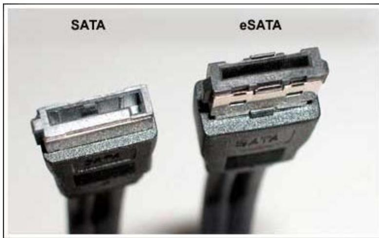
Figure 2. SATA and eSATA cable connectors.
