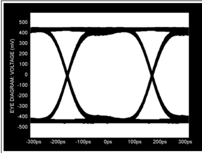
Figure 4. The MAX4951's eye pattern when operating at 3.0Gbps and an input of only 200mV<sub>P-P</sub>.
