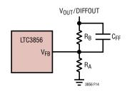
Figure 14. Setting Output Voltage without the DIFFAMP
