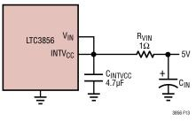
Figure 13. Set-Up for a 5V Input
