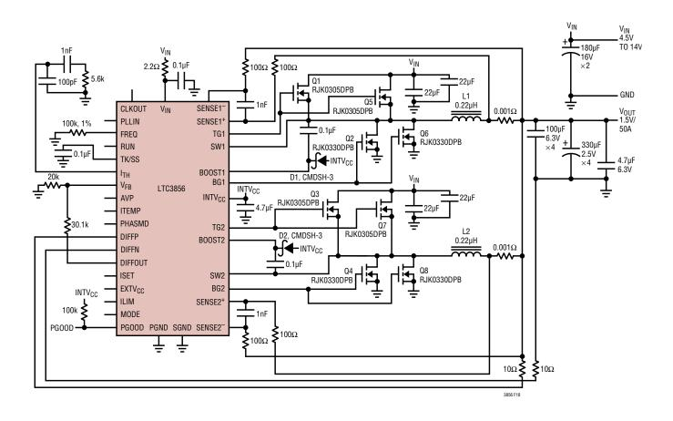
Figure 18. 1.5V/50A Converter Using Sense Resistors
