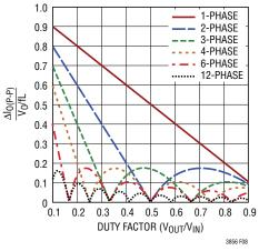
Figure 8. Normalized Peak Output Current vs Duty Factor [I<sub>RMS</sub> = 0.3(I<sub>OP-P</sub>)]
