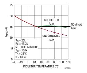
Figure 6. Worst Case  $I_{MAX}\xspace$  vs Inductor Temperature Curve with and without NTC Temperature Compensation
