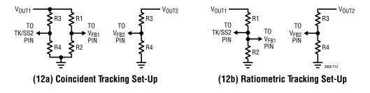
Figure 12. Set-Up and Coincident and Ratiometric Tracking
