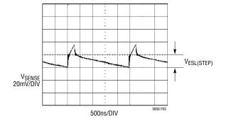
Figure 3. Voltage Waveform Measured Directly Across the Sense Resistor
