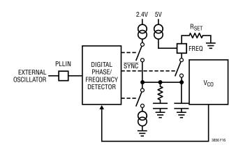
Figure 16. Phase-Locked Loop Block Diagram
