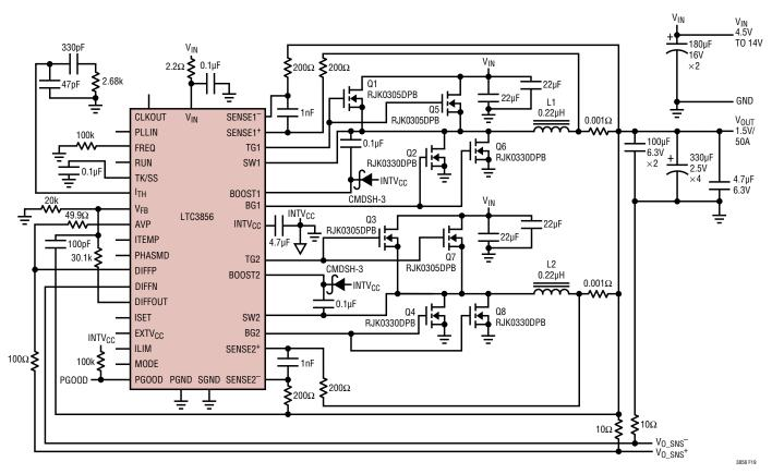
Figure 19. 1.5V/50A Converter with AVP
