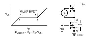
Figure 9. Gate Charge Characteristic
