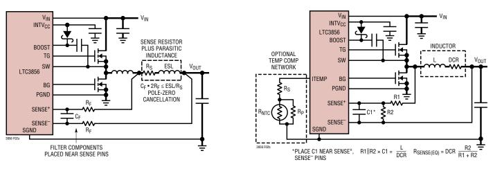
(2a) Using a Resistor to Sense Current
