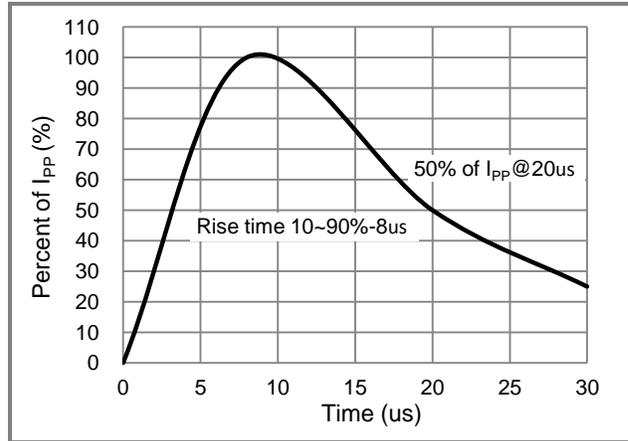
Fig.2 Pulse Waveform
