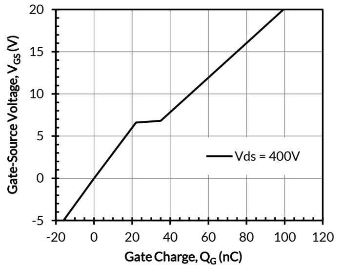
Figure 8. Typical gate charge at  $I_D = 60A$
