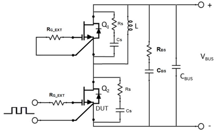
Figure 26. Schematic of the half-bridge mode switching test circuit. Note, a bus RC snubber ( $R_{BS} = 1\Omega$ ,  $C_{BS} = 100nF$ ) is used to reduce the power loop high frequency oscillations.
