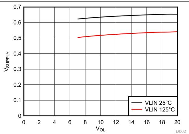
Figure 8-4.  $V_{OL}$  vs  $V_{SUPPLY}$  and Temperature
