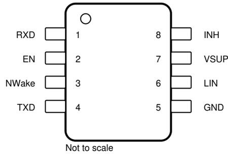
**Figure 7-1. D Package, 8-Pin SOIC (Top View)**
