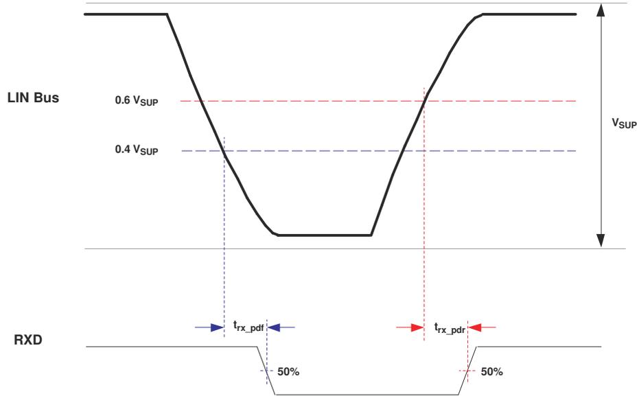
Figure 8-2. Propagation Delay
