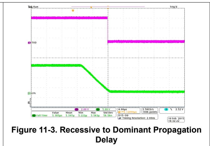
**Figure 11-3. Recessive to Dominant Propagation Delay**
