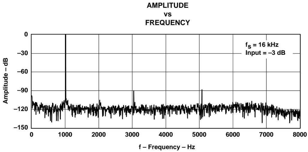
**Figure 5-4. FFT-ADC Channel**
