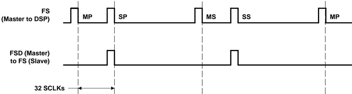
NOTE: MP: master primary (master-device data is transferred during this period, the DOUT of the slave device is in high-impedance state).
