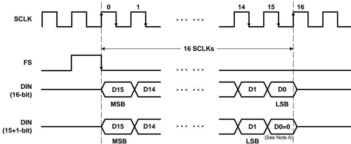
NOTE A: d0 = 0 means no secondary-communication request (software secondary-request control, see Section 3.2).
