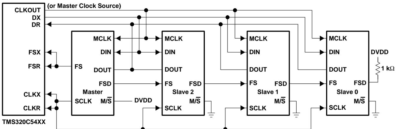
Figure 2–14. Cascade Mode Connection (to DSP Interface)
