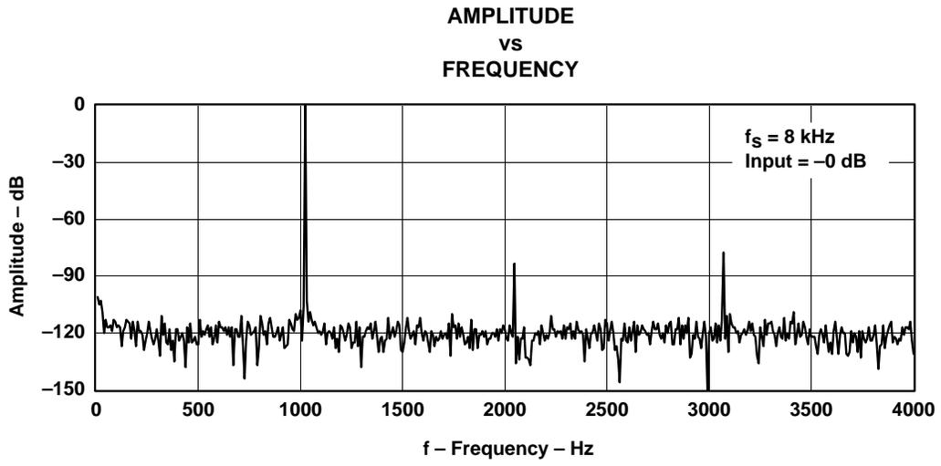
**Figure 5-9. FFT-DAC Channel**
