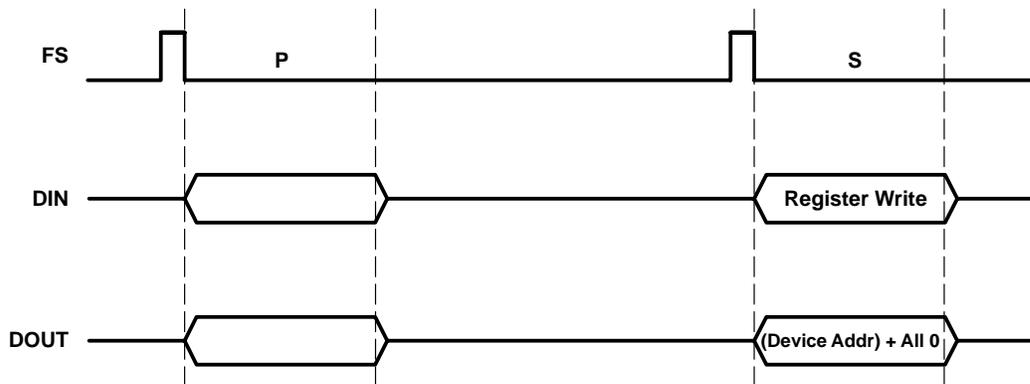
Figure 3–4. Device 3/Register 1 Write Operation Timing Diagram
