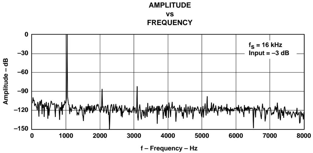
**Figure 5-6. FFT-DAC Channel**
