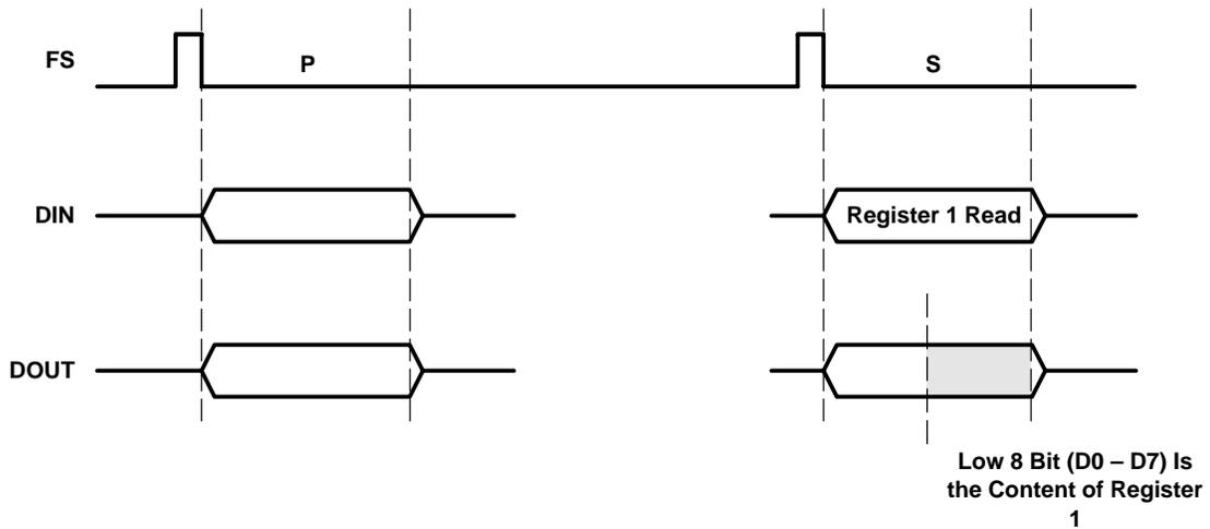
Figure 3–3. Device 3/Register 1 Read Operation Timing Diagram
