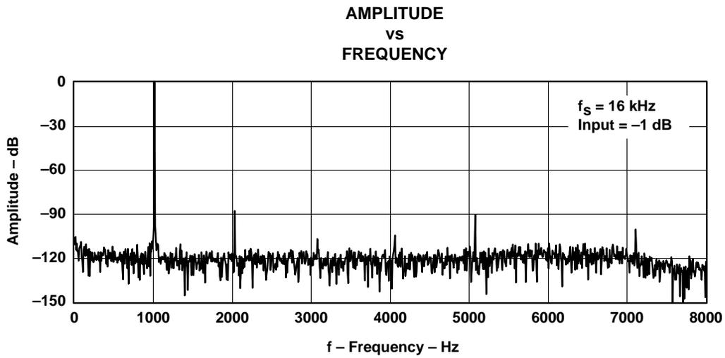
**Figure 5-8. FFT-ADC Channel**
