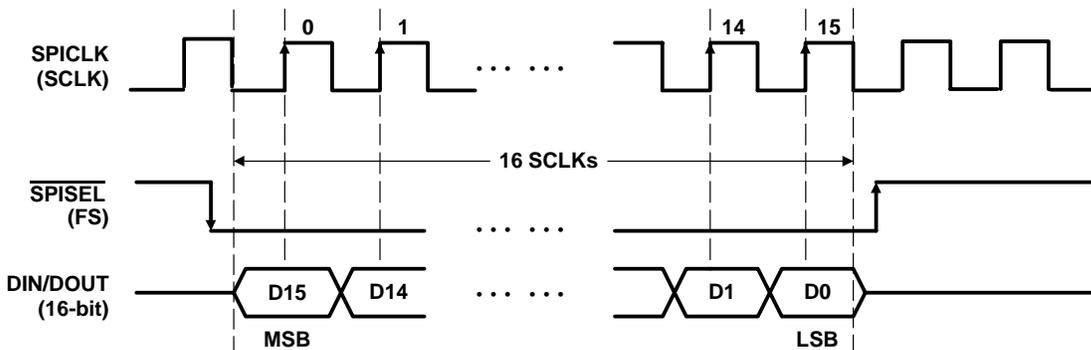
**Figure 2–10. Timing Diagram for the SPI\_CP1 Mode (M1M0 = 10)**
