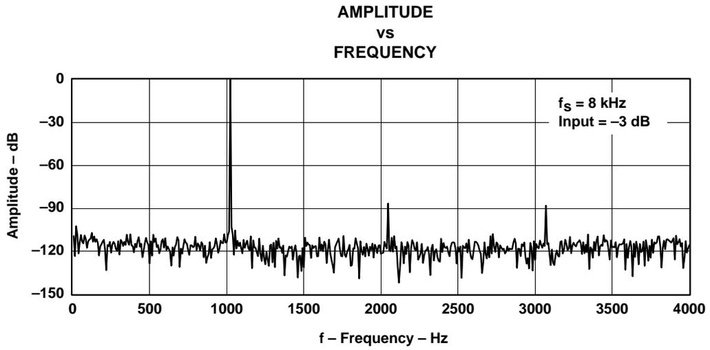
**Figure 5-5. FFT-DAC Channel**
