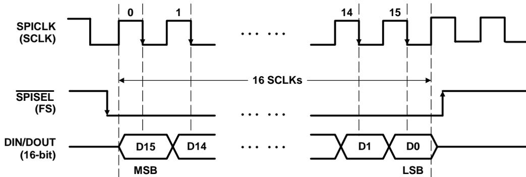
**Figure 2–9. Timing Diagram for the SPI\_CP0 Mode (M1M0 = 01)**
