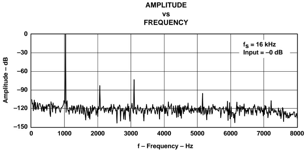
**Figure 5-10. FFT-DAC Channel**
