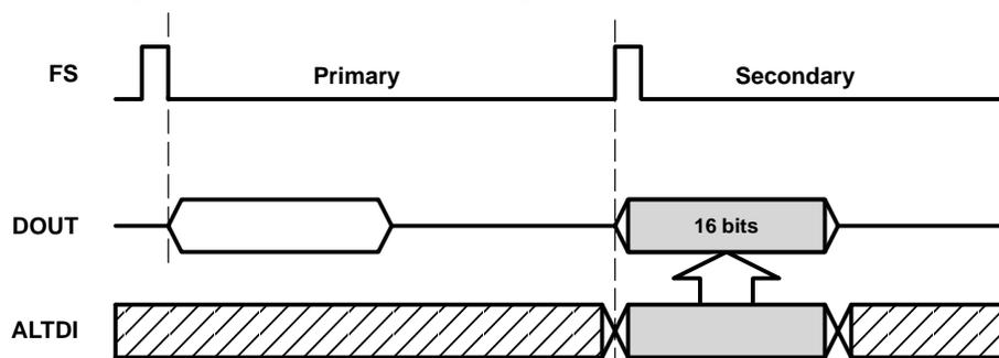
NOTE A: When DIN performs a write operation (sets D12 to 0) during secondary communication.
