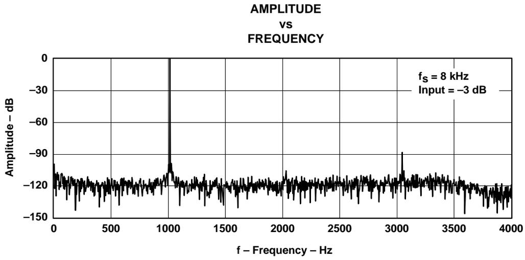
**Figure 5-3. FFT-ADC Channel**
