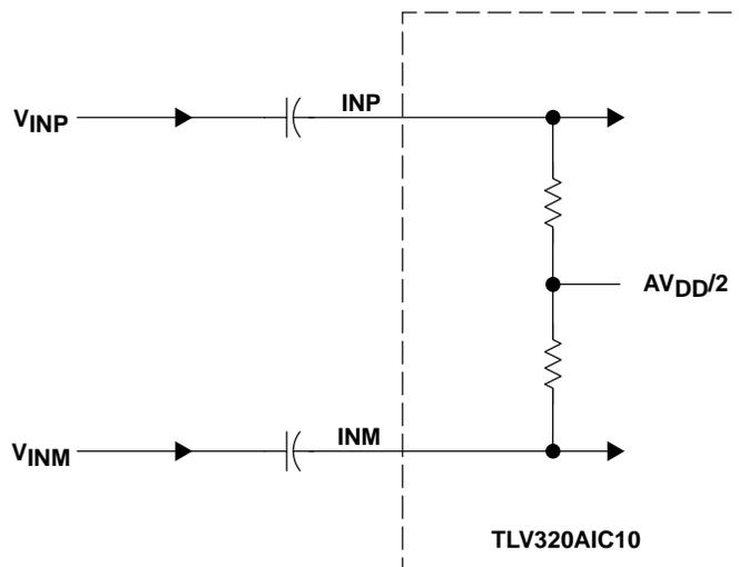
Figure 2–16. INP and INM Internal Self-Biased ( $AV_{DD}/2$ ) Circuit
