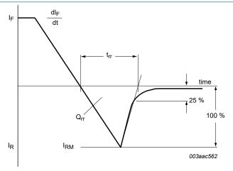
Fig. 15. Reverse recovery definition; ramp recovery
