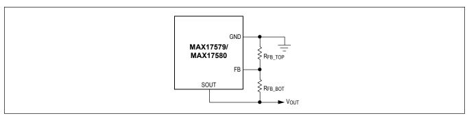
Figure 2. Setting the Output Voltage
