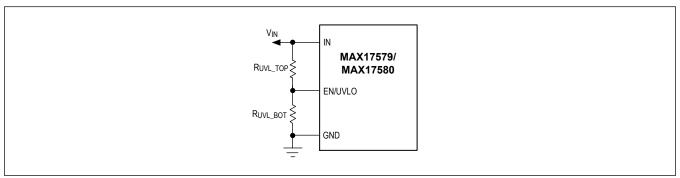
Figure 3. Setting the Input Undervoltage-Lockout
