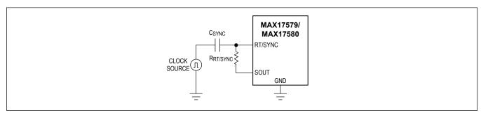
Figure 1. Synchronization to an External Clock
