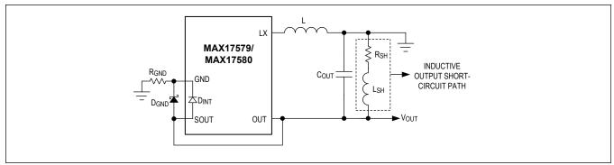
Figure 4. Inductive Output Short-Circuit Protection
