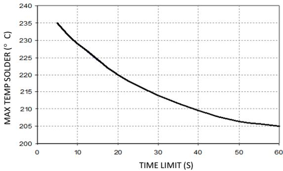
Figure 22. Time Limit, T<sub>lim</sub>, Curve Above 205°C Reflow.
