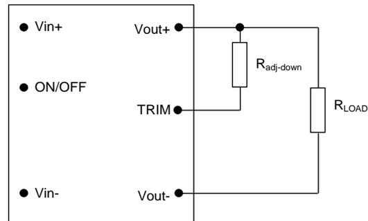
**Figure 11. Circuit Configuration to Decrease Output Voltage.**
