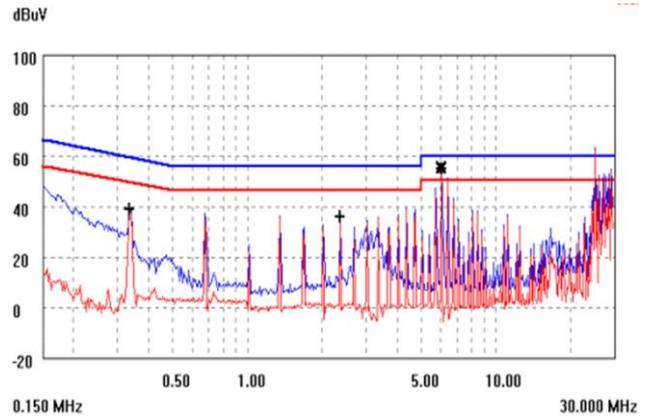
**Figure 19. EMC signature using above filter, SHHDA.**
