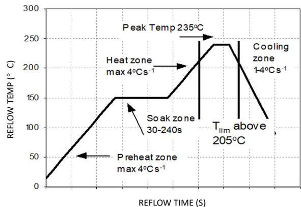
Figure 21. Recommended Reflow Profile for Sn/Pb solder.
