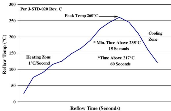
Figure 23 Recommended linear reflow profile using Sn/Ag/Cu solder.
