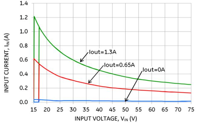
Figure 2. Converter Input Current versus Input Voltage.
