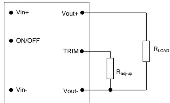
**Figure 12. Circuit Configuration to Increase Output Voltage.**
