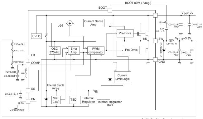
C1,C8,C5,C9 = Ceramic capacitor L1=CDRH105RNP-100NC(sumida)
