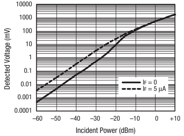
**Figure 7. Detector Voltage @ 2.45 GHz (100 kΩ Video Resistance)**
