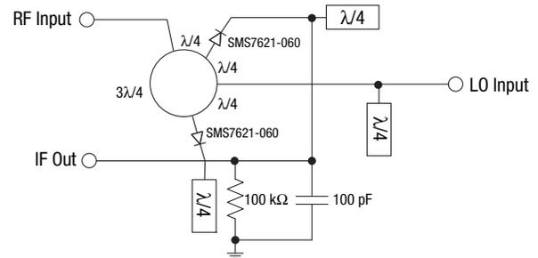
Figure 4. Schematic of a 24 GHz Rat-Race Mixer
