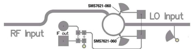
Figure 5. Layout for a 24 GHz Rat-Race Mixer
