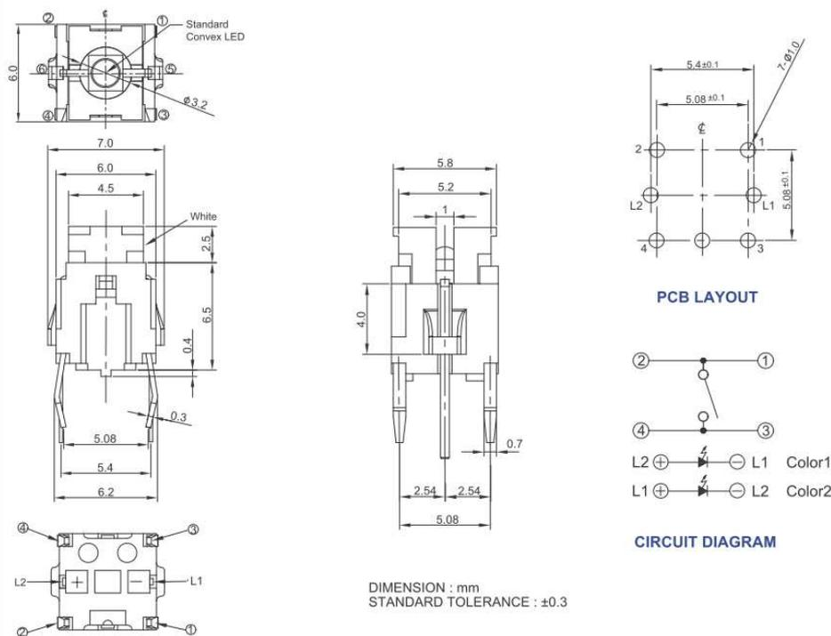
Figure 2 – 228BMV, Surface Mount Gull Wing, Vertical Actuation
