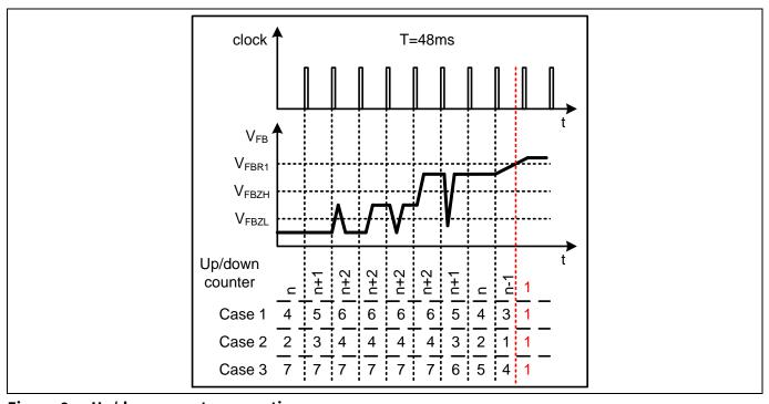
Figure 6 Up/down counter operation
