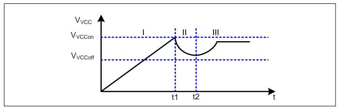
Figure 4 VCC voltage at start up
