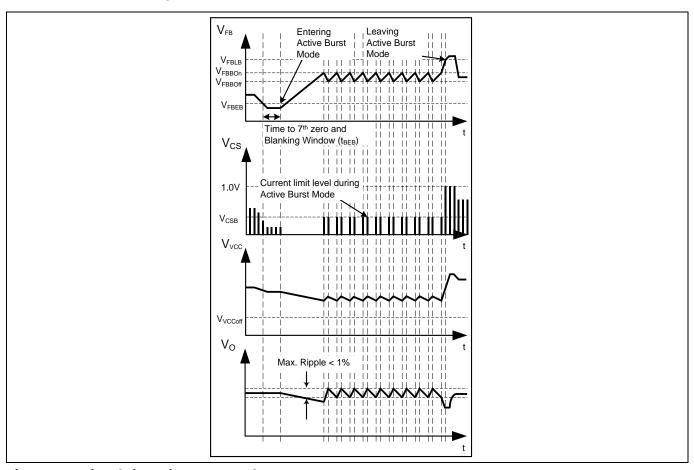
Figure 9 **Signals in Active Burst Mode**
