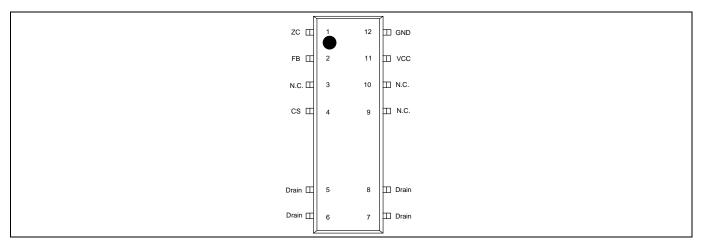
Figure 2 Pin configuration PG-DSO-12(top view)
