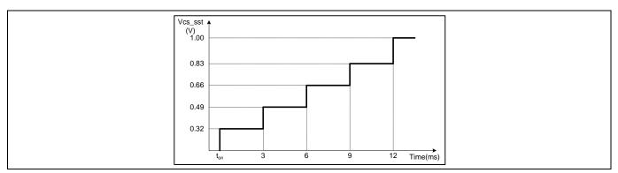
Figure 5 Maximum current sense voltage during soft start
