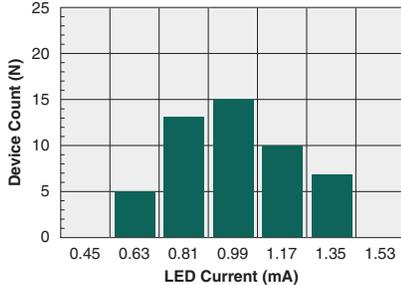
Typical  $I_F$  for Switch Dropout
