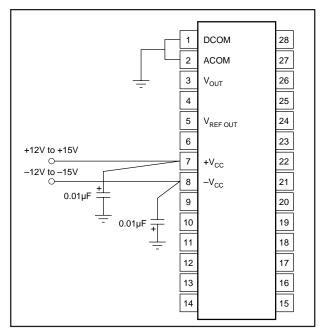
FIGURE 4. Power Supply Connections.
