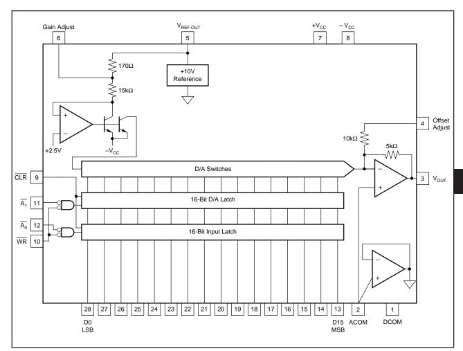
FIGURE 1. DAC715 Block Diagram.
