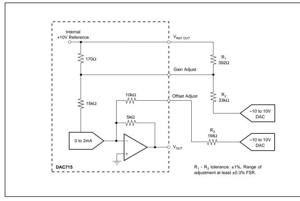
FIGURE 7. Gain and Offset Adjustment Using D/A Converters.
