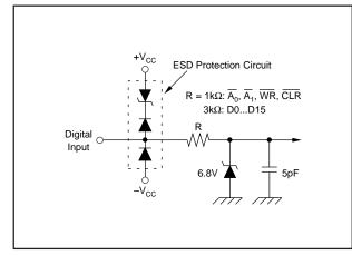
FIGURE 2. Equivalent Circuit of Digital Inputs.
