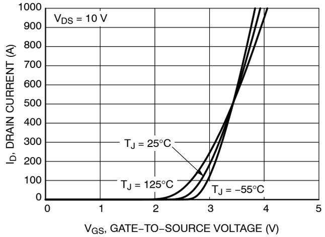
Figure 2. Transfer Characteristics
