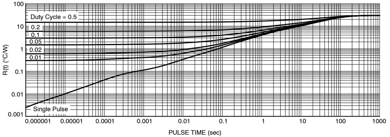
Figure 13. Thermal Characteristics
