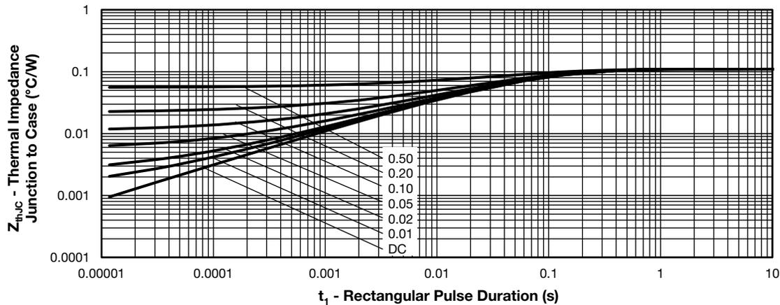
Fig. 4 - Maximum Thermal Impedance  $Z_{thJC}$  Characteristics
