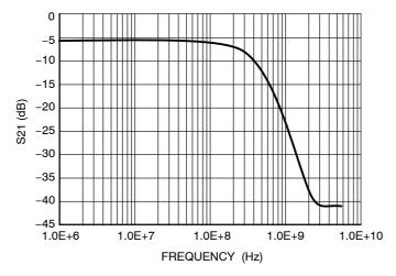
Figure 4. Insertion Loss Characteristic
