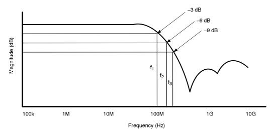
Figure 7. Filter Bandwidth
