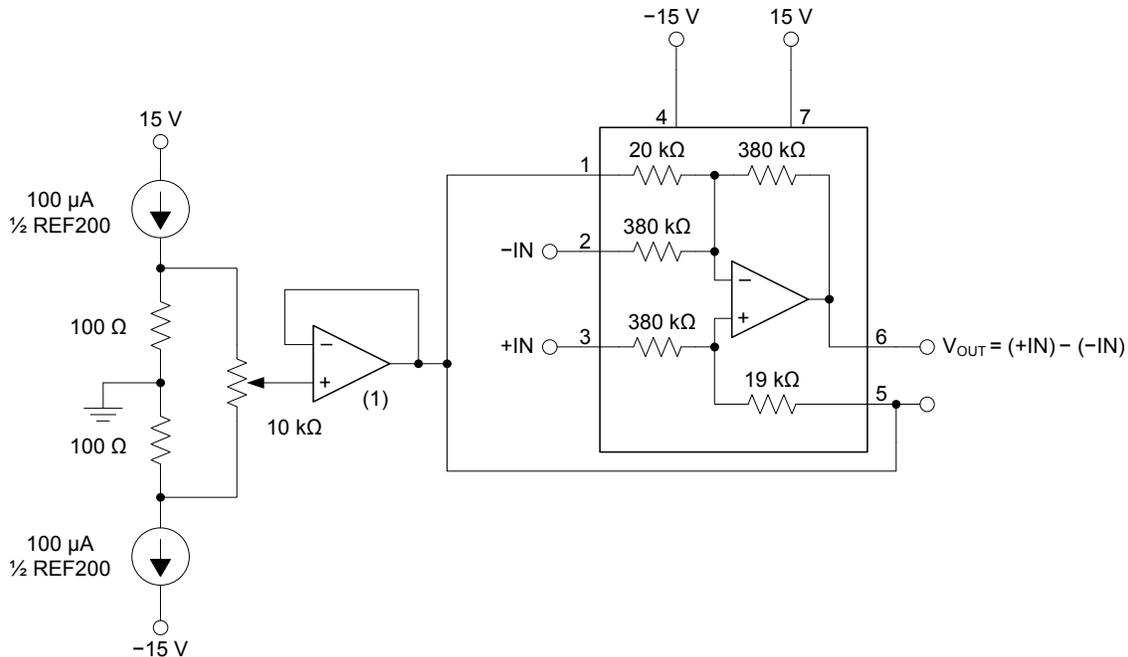
(1) The OPA171 (a 36-V, low-power, RRO, general-purpose operational amplifier) can be used for this application.
