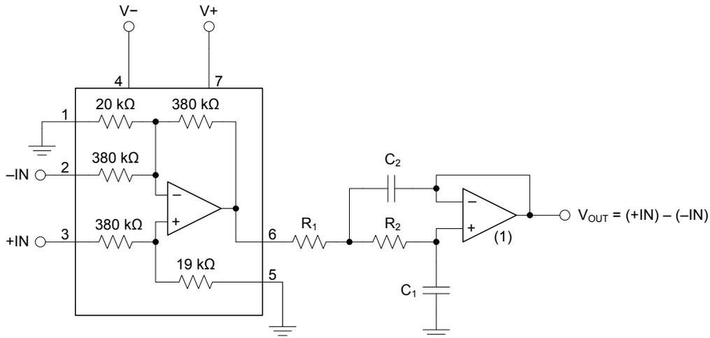
(1) For most applications, the OPA171 can be used as an operational amplifier. For directly driving successive-approximation register (SAR) data converters, the OPA140 is a good choice.
