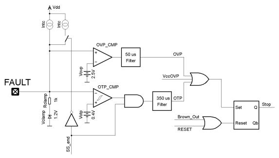
Figure 74. OVP/OTP Detection Schematic
