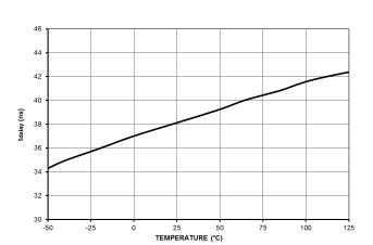
Figure 11. Propagation Delay t<sub>delay</sub>
