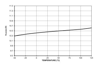
Figure 29. HV Current Source Restart Threshold  $V_{\text{CC(min)}}$
