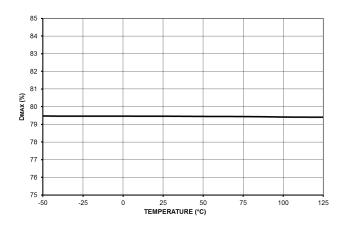
Figure 23. Maximum Duty Cycle  $D_{\mbox{\scriptsize MAX}}$
