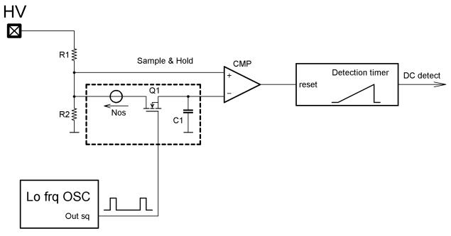
Figure 51. The ac Line Unplug Detector Structure Used for X2 Capacitor Discharge System
