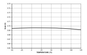
Figure 9. Maximum Internal Current Setpoint  $V_{\text{ILIM}}$
