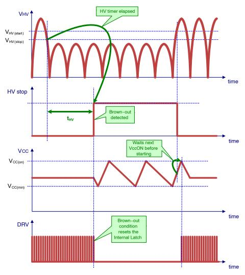
Figure 48. Ac Line Drop-out Timing Diagram
