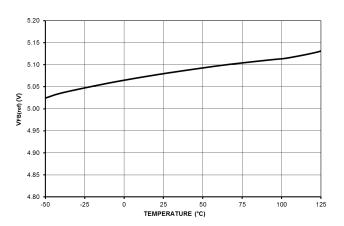
Figure 18. FB Pin Open Voltage V<sub>FB(ref)</sub>
