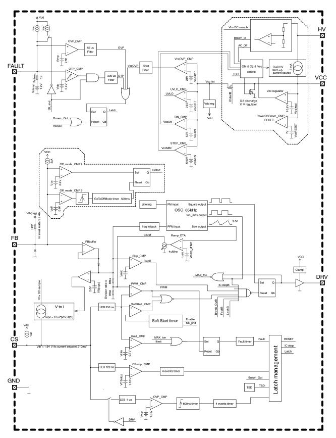
Figure 2. Simplified Internal Block Schematic
