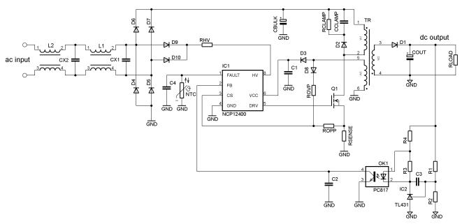
Figure 1. Flyback Converter Application using the NCP12400
