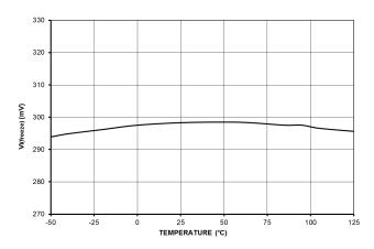
Figure 12. Frozen Current Setpoint  $V_{I(freeze)}$  for the Light Load Operation
