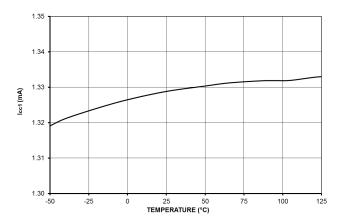
Figure 28. Internal Current Consumption when DRV Pin is Unloaded  $I_{\text{CC1}}$
