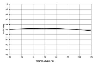
Figure 4. High Voltage Startup Current Flowing Out of  $V_{CC}$  Pin  $I_{start1}$  of  $V_{CC}$  Pin Fault/Short
