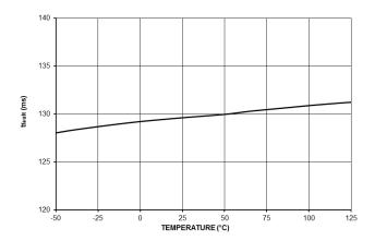
Figure 24. The Fault Timer Duration t<sub>fault</sub>
