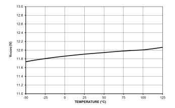
Figure 26.  $V_{CC}$  Turn-on Threshold Level,  $V_{CC}$  Going Up HV Current Source Stop Threshold  $V_{CC(on)}$
