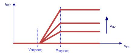
Figure 68. Overpower Protection Current Relation to Feedback Voltage
