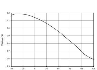
Figure 22. X2 Discharge Comparator Hysteresis Observed at HV Pin V<sub>HV(hyst)</sub>
