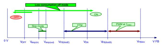
Figure 43. Mode Control with FB Pin Voltage
