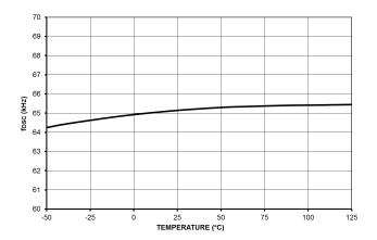
Figure 20. Oscillator Switching Frequency fosc
