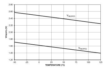
Figure 37. FB Pin Voltage Thresholds for Overpower Compensation
