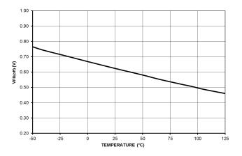
Figure 16. Built in Offset between FB Pin and Internal Divider V<sub>FB(off)</sub>
