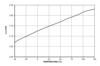
Figure 31. Internal Current Consumption when DRV Pin is Loaded by 1 nF Capacitance I<sub>CC2</sub>
