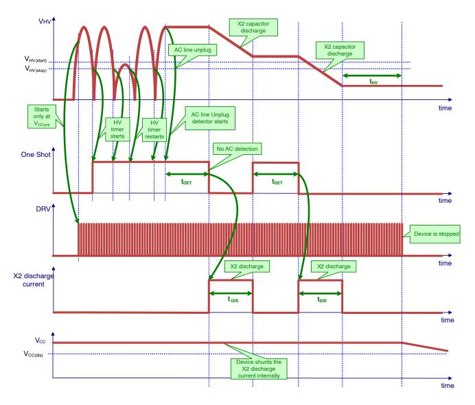
Figure 55. HV Pin ac Input Timing Diagram with X2 Capacitor Discharge Sequence When the Application is Unplugged Under High Line Condition
