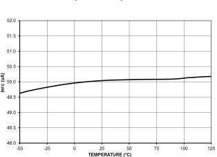
Figure 39. Current I<sub>NTC</sub> Sourced Out from the Fault Pin, allowing Direct NTC Connection
