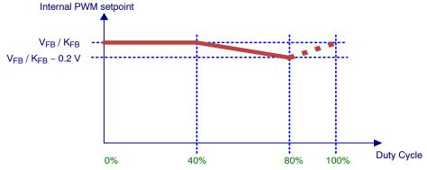
Figure 66. Slope Compensation Timing Diagram
