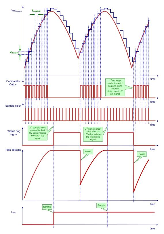
Figure 71. Overpower Compensation Timing Diagram
