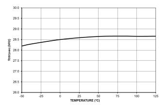
Figure 21. Minimum Switching Frequency fosc(min)
