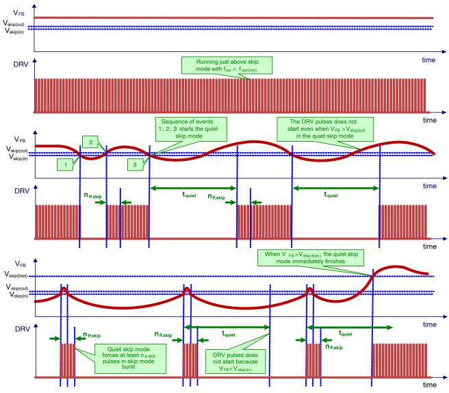
Figure 63. Quiet-Skip Timing Diagram - option
