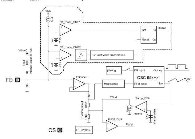
Figure 65. Slope Compensation Block Diagram
