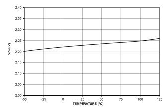
Figure 33. FB Pin Voltage Level Above which is Entered Normal Operating Mode  $V_{ON}$
