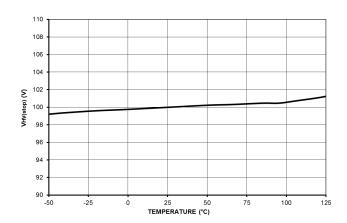
Figure 8. HV Pin Device Stop Threshold V<sub>HV(stop)</sub>
