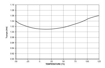
Figure 25. HV Signal Sampling Period T<sub>sample</sub>
