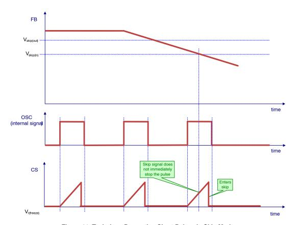
Figure 61. Technique Preventing Short Pulses in Skip Mode
