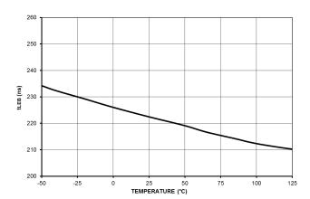
Figure 14. Leading Edge Blanking Duration t<sub>LEB</sub>
