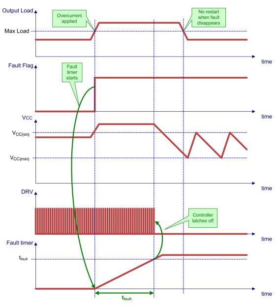
Figure 72. Latched Timer-Based Overcurrent Protection
