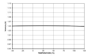
Figure 13. Over Voltage Protection Threshold at CS Pin  $V_{\rm OVP(CS)}$
