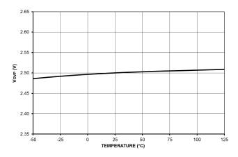
Figure 38. Fault Pin High Threshold for OVP  $V_{OVP}$
