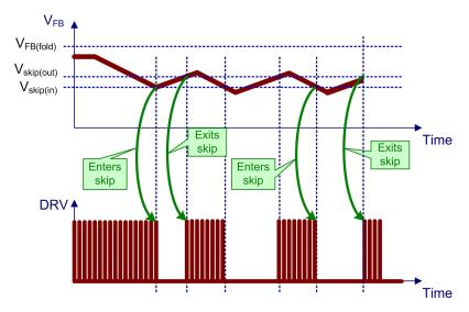
Figure 60. Skip Mode Timing Diagram
