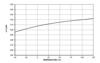
Figure 32. Internal Current Consumption in Skip Mode I<sub>CC3</sub>
