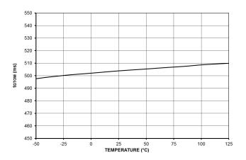
Figure 34. Go To Off Mode Timer Duration  $t_{\mbox{\scriptsize GTOM}}$
