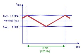
Figure 57. Frequency Modulation of the Maximum Switching Frequency
