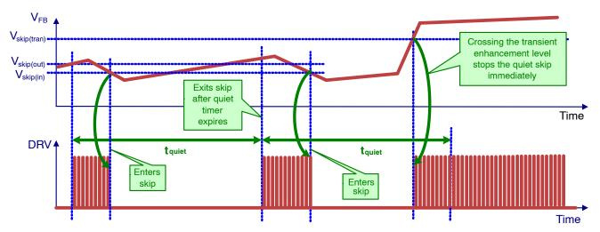
Figure 62. Leaving the Quiet-Skip Mode during Load Transient
