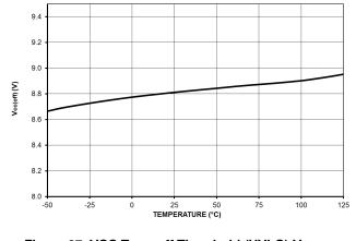
Figure 27. VCC Turn-off Threshold (UVLO) V<sub>CC(off)</sub>
