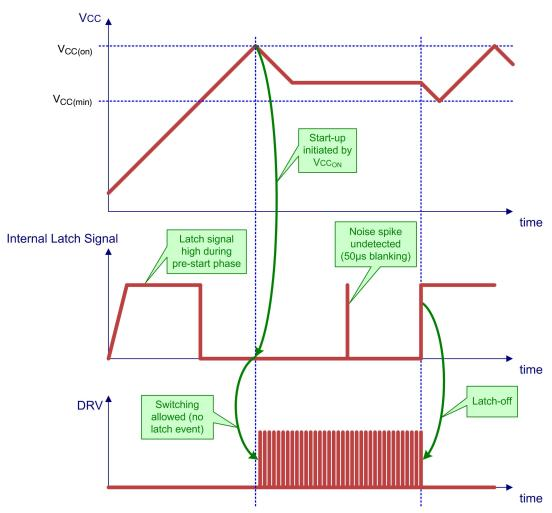
Figure 75. Latch Timing Diagram
