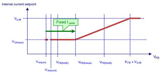
Figure 59. Current Setpoint Dependency on the Feedback Pin Voltage
