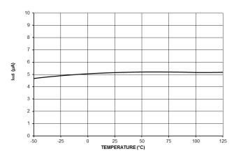
Figure 35. Internal Current Consumption in Off Mode  $I_{CC5}$
