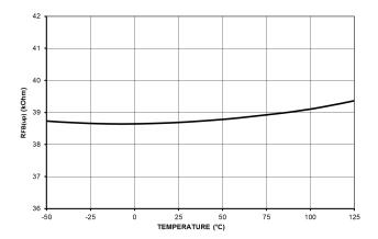
Figure 15. FB Pin Internal Pull-up Resistor  $R_{FB(up)}$
