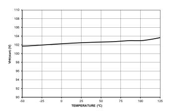
Figure 5. HV Pin Device Startup Threshold  $V_{HV(start)}$
