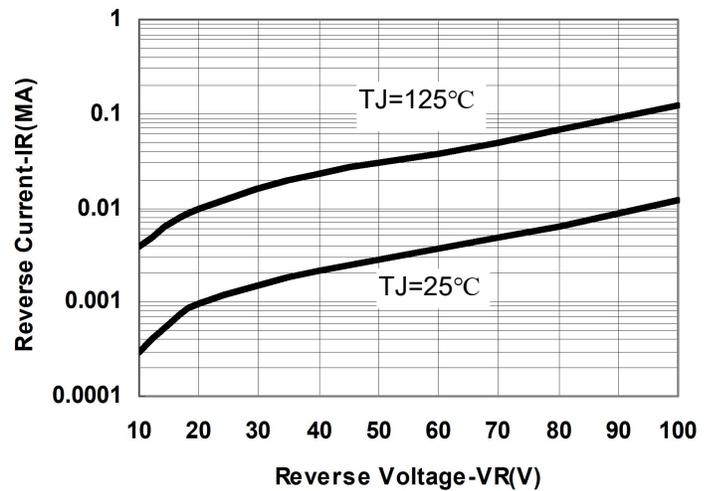
Fig.2-Typical Reverse Current
