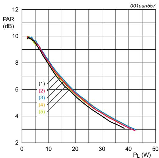
$V_{DS} = 28\text{ V}; I_{Dq} = 450\text{ mA}.$
