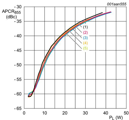
$V_{DS} = 28\text{ V}; I_{Dq} = 450\text{ mA}.$
