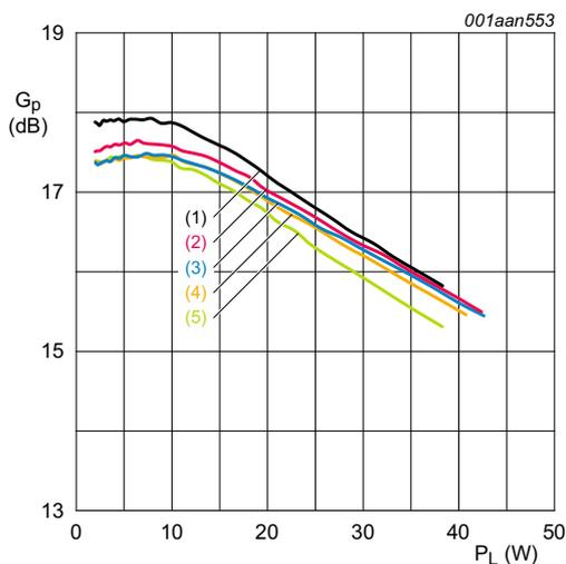
$V_{DS} = 28$  V;  $I_{Dq} = 450$  mA.
