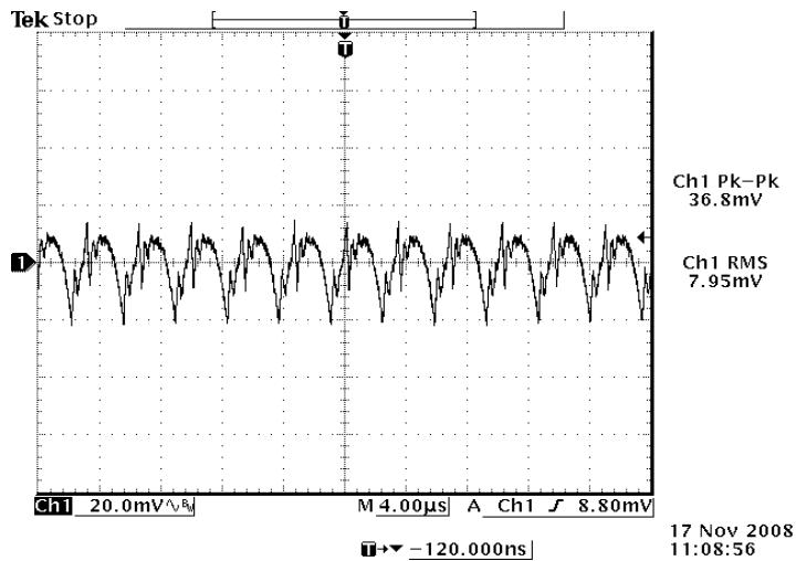
75Vdc input, 1.2Vdc/50A output
