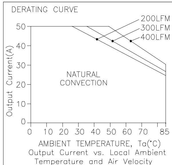
Vin=48V, with maximum junction temperature of semiconductors derated to 120C
