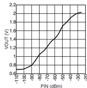
**Figure 9. Typical RSSI Characteristics**
