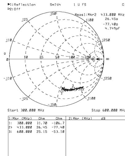
Figure 8. Input Impedance
