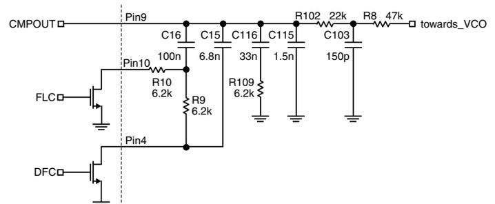
**Figure 7. Dual-Loop Filters**
