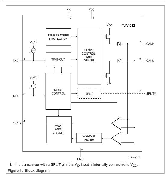
High-speed CAN transceiver with Standby mode
