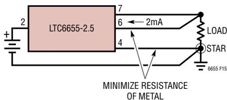
Figure 16. Kelvin Connection for Good Load Regulation
