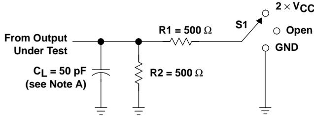
NOTE: When  $V_{CC} = 1.5 \text{ V}$ ,  $R_1$  and  $R_2 = 1 \text{ k}\Omega$ .
