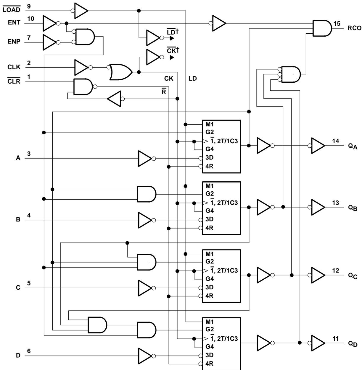
† For simplicity, routing of complementary signals  $\overline{LD}$  and  $\overline{CK}$  is not shown on this overall logic diagram. The uses of these signals are shown on the logic diagram of the D/T flip-flops.
