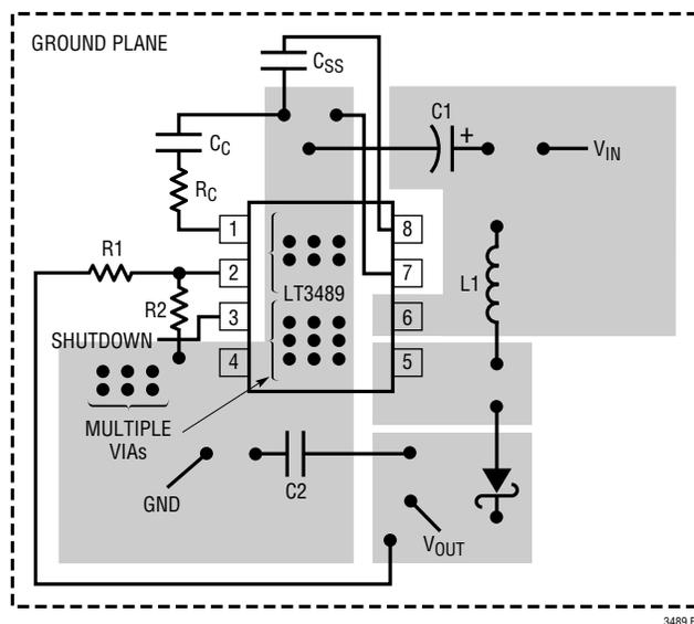
**Figure 2. Recommended Component Placement for Boost Converter. Note Direct High Current Paths Using Wide PC Traces. Minimize Trace Area at Pin 1 ( $V_C$ ) and Pin 2 (FB). Use Multiple Vias to Tie Pin 4 Copper to Ground Plane. Use Vias at One Location Only to Avoid Introducing Switching Currents Into the Ground Plane**
