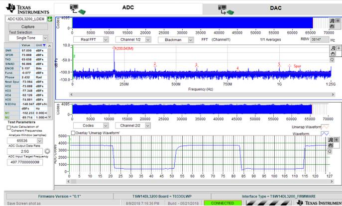
Figure 178. 200-MHz, Sine-Wave (Channel A) Frequency Domain (FFT) and 40-MHz, Square-Wave (Channel B) Time Domain for 5-GSPS, Single-Channel Oscilloscope
