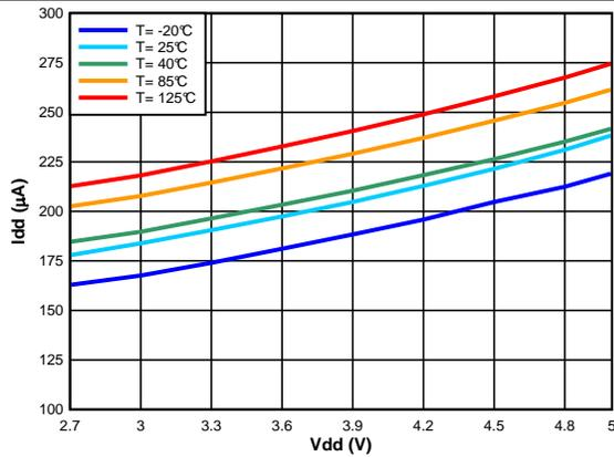
Figure 4. Supply Current vs. Supply Voltage, RH Measurement
