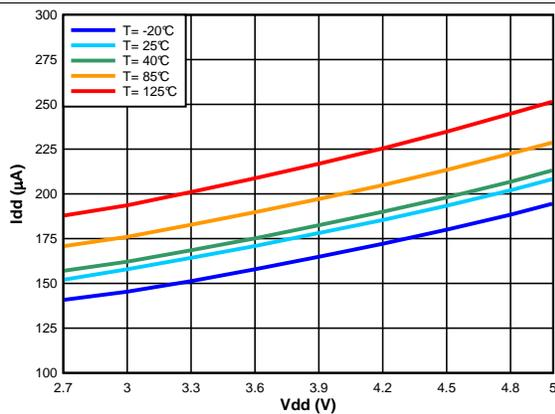
Figure 6. Supply Current vs. Supply Voltage, Temp Measurement
