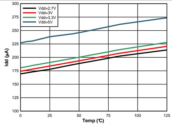
Figure 5. Supply Current vs. Temperature, RH Measurement
