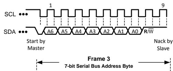
**Figure 13. Read Humidity/Temperature Measurement (Data Not Ready)**
