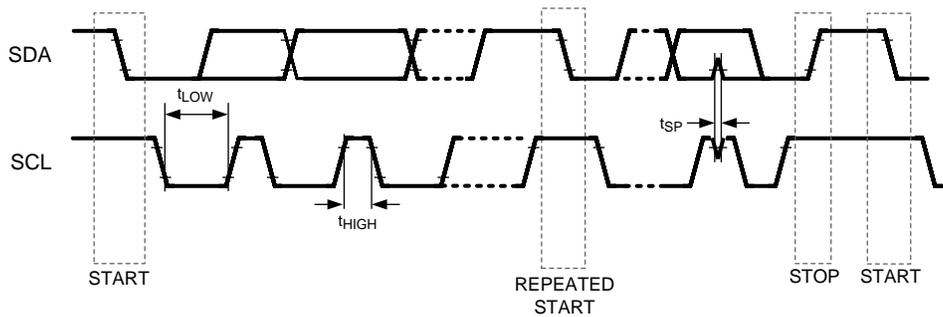
Figure 1. I<sup>2</sup>C Timing
