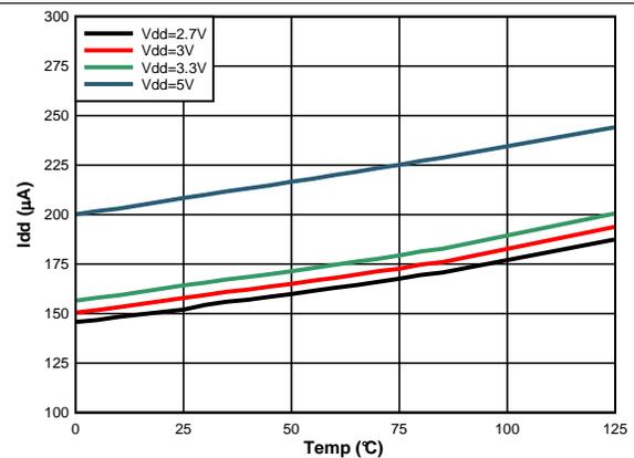
Figure 7. Supply Current vs. Temperature, Temp Measurement
