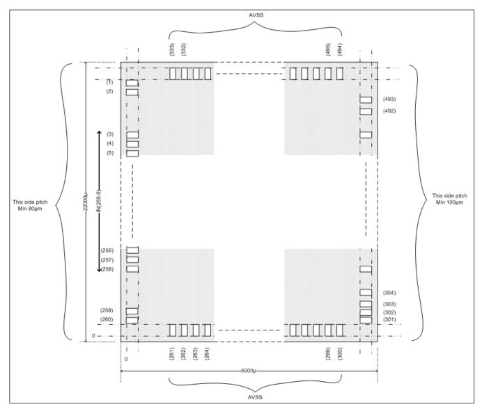
Figure 2. GBTD Die Mechanical Data
