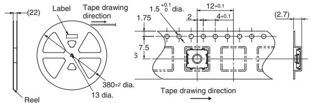
100 packing reel for packing (B3SE-1002P-R100)
