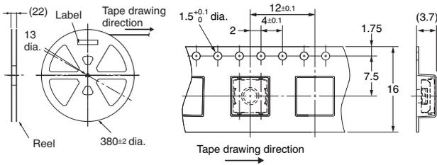
100 packing reel for packing (B3FS-100□P-R100)
