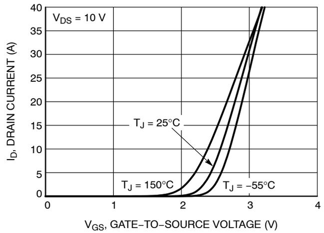
Figure 2. Transfer Characteristics
