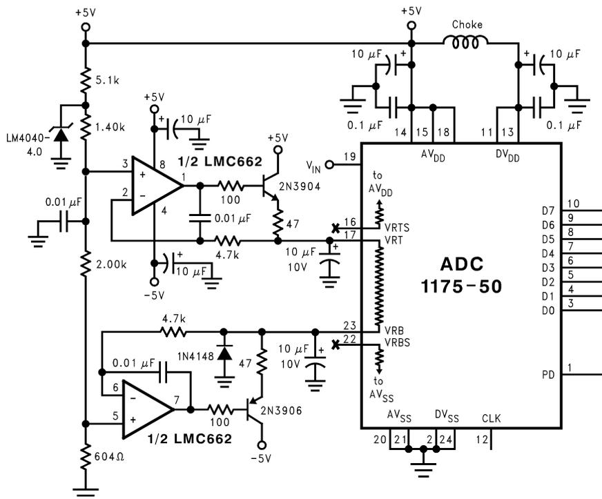
Requires driving with a low impedance source, provided by the transistors. Note that pins 16 and 22 are not connected.
