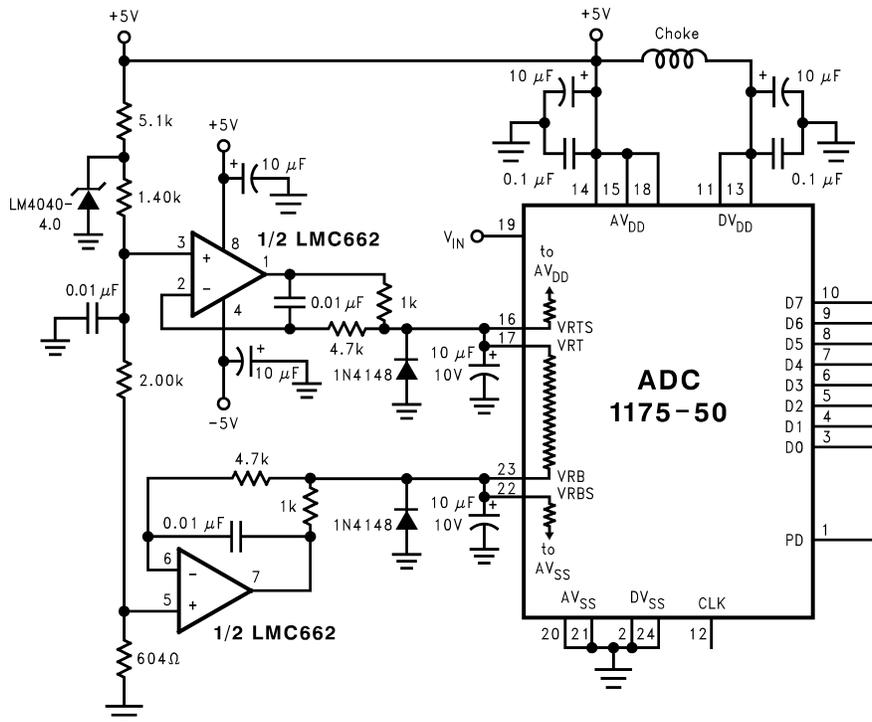
Self bias is still used, but the reference voltages are trimmed by providing a small trim current with the operational amplifiers.
