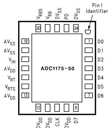
**Figure 2. 24-Pin WQFN - Bottom View**
