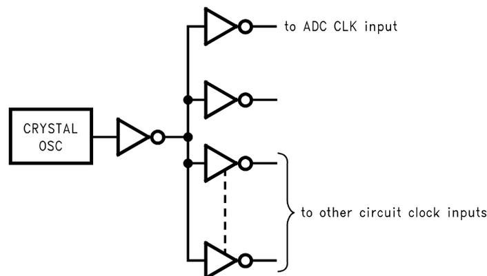
**Figure 20. Isolating the ADC Clock from Digital Circuitry**
