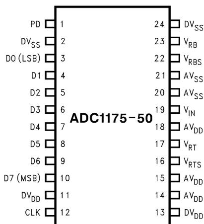
**Figure 1. 24-Pin TSSOP - Top View**
