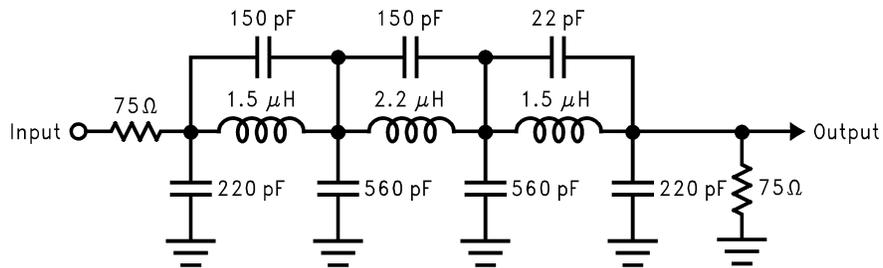
Use with maximum input frequencies of 1 MHz to 5 MHz.
