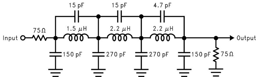
Use with maximum input frequencies of 5 MHz to 10 MHz.
