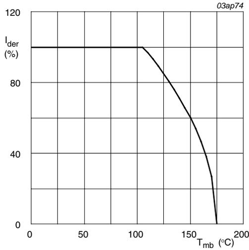
$$I_{der} = \frac{I_D}{I_{D(25^\circ\text{C})}} \times 100\%$$
