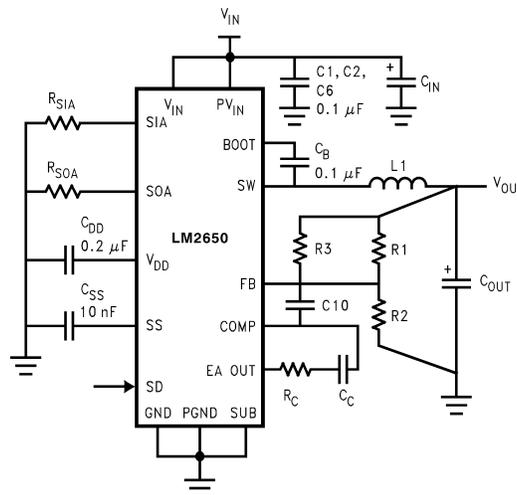
Figure 18. The Typical 90 kHz Application Circuit
