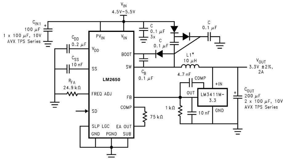
**Figure 19. An Efficient, 2% Accurate 5V to 3.3V Converter**
