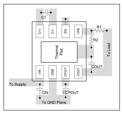
Figure 23. LM27761 Layout Example
