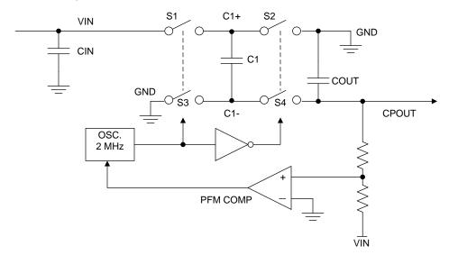
Figure 17. Voltage Inverting Principle
