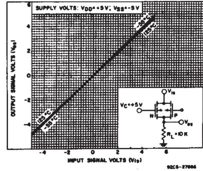
Fig. 7—Typ. on-state characteristics as a function of temp. for 1 of 4 switches with V<sub>DD</sub> = +5 V, V<sub>SS</sub> = -5 V.
