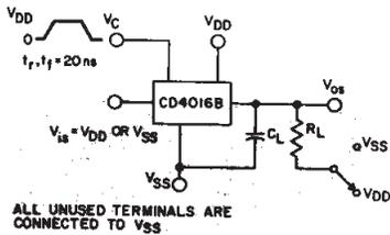
Fig. 25 - Turn-On propagation delay-control input.
