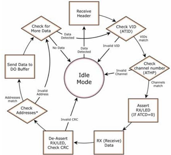
Note: If serial data exists in the DI buffer while the module is in Receive Mode, the UART data will be transmitted after the module is finished receiving the RF data and has returned to Idle Mode.
