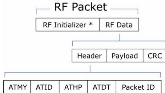
\* When streaming multiple RF packets, the RF Initializer is only sent in front of the first packet.
