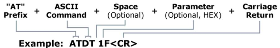
The preceding example would change the module Destination Address to “0x1F”. For modified parameter values to persist in the module registry, changes must be saved to non-volatile memory using WR (Write) Command. Otherwise, parameters are restored to previously saved values after the module is powered off and then on again.
