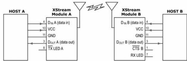
The data flow sequence is initiated when the first byte of data is received in the DI Buffer of the transmitting module (XStream Module A). As long as XStream Module A is not already receiving RF data, data in the DI Buffer is packetized, then transmitted over-the-air to XStream Module B-0
