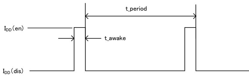
The Hall IC is operated intermittently to reduce supply current.
