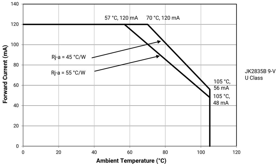
**FLUX CHARACTERISTICS, ORDER CODES AND BINS - JK2835B 9-V U CLASS ( $I_F = 100 \text{ mA}$ ,  $T_j = 25 \text{ °C}$ )**
