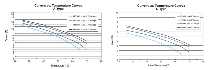
The above curves were derived from placing test samples in an oven at 25  $^{\circ}$ C, 40  $^{\circ}$ C, 60  $^{\circ}$ C and 70  $^{\circ}$ C, increasing current flow through the sample at a rate of 0.1 A/minute and recording the current value when the sample trips.
