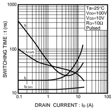
Fig.13 Switching Characteristics
