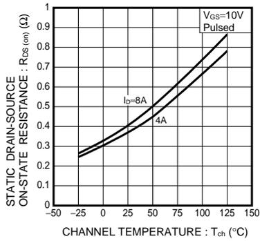
Fig.7 Static Drain-Source On-State Resistance vs. Channel Temperature
